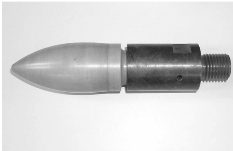
Figure 11: Mandrel made of ceramics and adapter used with cross-roll piercing of copper
