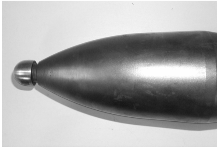
Figure 7: Special mandrel for measuring tip force
